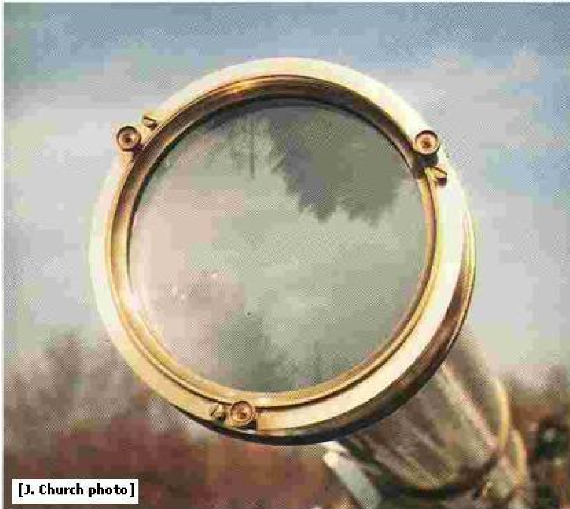
The Hastings 6-1/4 inch objective in its cell and tube by John Byrne (1879-80)
